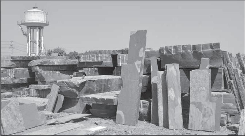
The blocks thus split are transported to other areas of mine or to a stock place for further splitting into slabs of required length.
