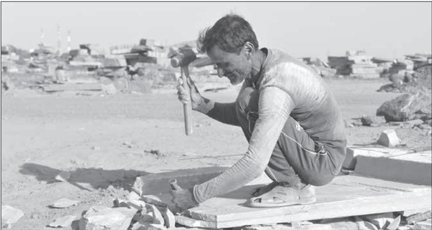
Layers in the sandstone block are obtained by the same technique as preparing the block for excavation - by constantly hammering the block. Layers of block are then cut into marked sizes using chisels.
