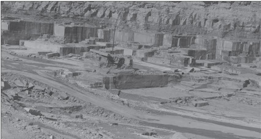
The hard and non-splittable sandstone block locally known as *Bhaata* is then drilled and blasted to expose the underlying sandstone. Debris from blasting and the *bhaata* is then removed from the mine site over a period of 2 days and the initial quarrying begins. Clearing of debris and top soil is categorised as unskilled work and generally carried out by women. Women do none of the “skilled” work in the sandstone mines.
